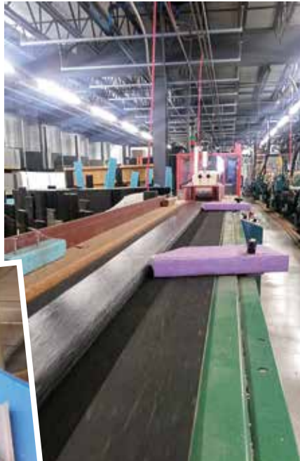
High Density Polyethylene extrusion line.
